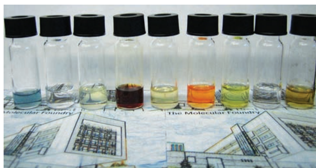
Figure 5. Dispersions of \text{BF}_4^- /DMF passivated nanocrystals. From left to right: ITO, AZO, \text{TiO}_2 , \alpha\text{-Fe}_2\text{O}_3 , CdSe/ZnS ( \lambda_{\text{em}} = 545 \text{ nm} ), CdSe/ZnS ( \lambda_{\text{em}} = 605 \text{ nm} ), CdSe/CdS quantum dot/quantum rods ( \lambda_{\text{em}} = 619 \text{ nm} ), upconverting \text{NaYF}_4\text{:Yb/Tm} , and Ag nanocrystals.
